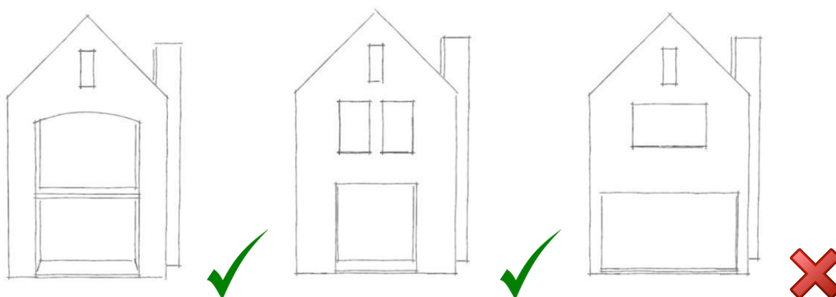
Fig 16-18: Large vertical proportioned windows & punched openings encouraged.
